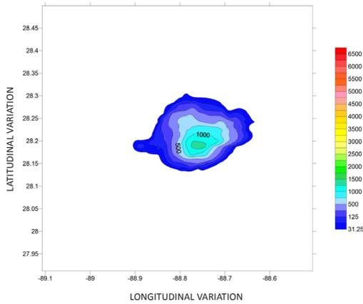
**Figure 3C.** BTEX field (ppb) at 750 m, with dispersants.
