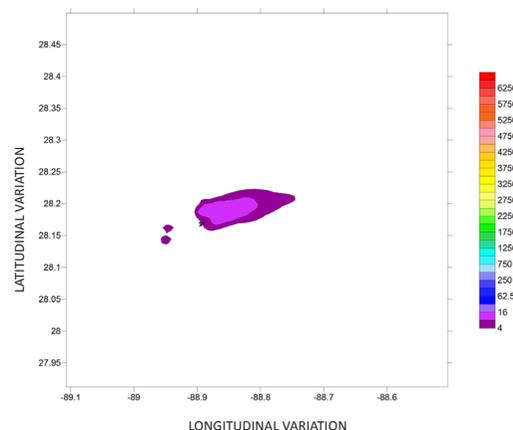
**Figure 3B.** BTEX field (ppb) at 1200 m, without dispersants.
