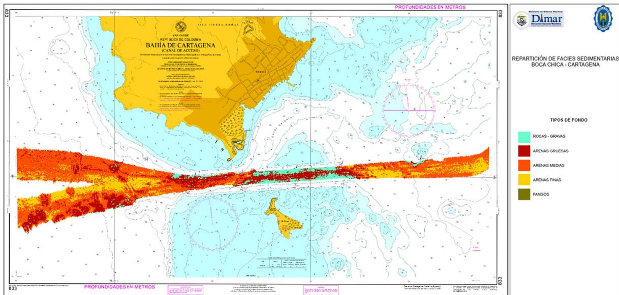
**Figure 10.** Characterization of funds using backscatter technology.
