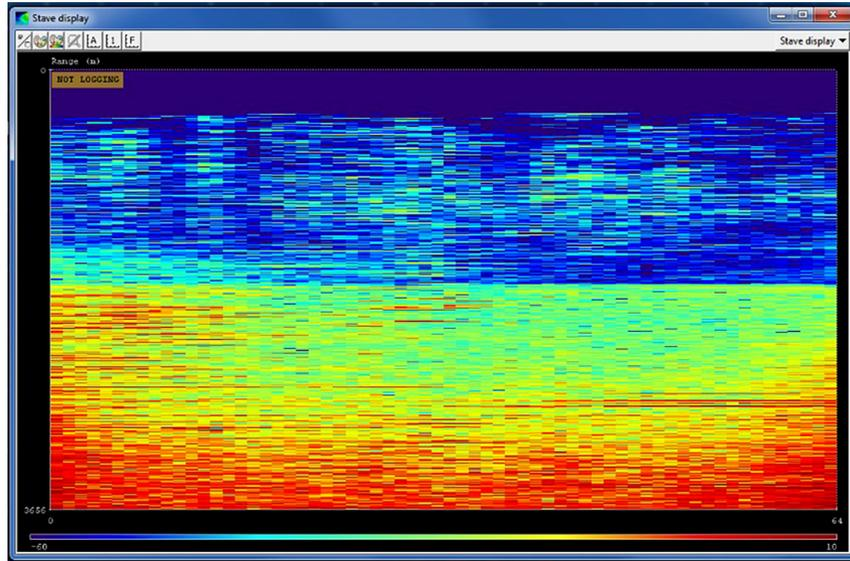
**Figure 6.** Stave display during the test at a depth of 1739m, speed 8.1knt and heading 088T.
