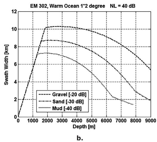
**Figure 3.** Performance of the different arrangements of the Kongsberg EM 302 echo sounders in the oceanographic vessels of the CIOH-Caribe: a) ARC Providencia b) ARC Malpelo. Source: Kongsberg Maritime AS.
