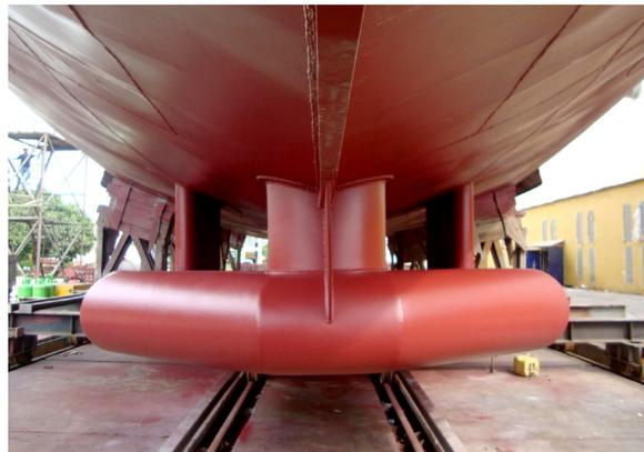
**Figure 2.** Gondola of the arrangement of sensors of the multibeam systems in the lower part of the hull of the vessels ARC Malpelo and ARC Providencia.
