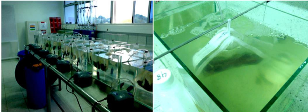
**Figura 3.** Experimental set-up of bioassays for the removal of BOD<sub>5</sub> and TVS.
