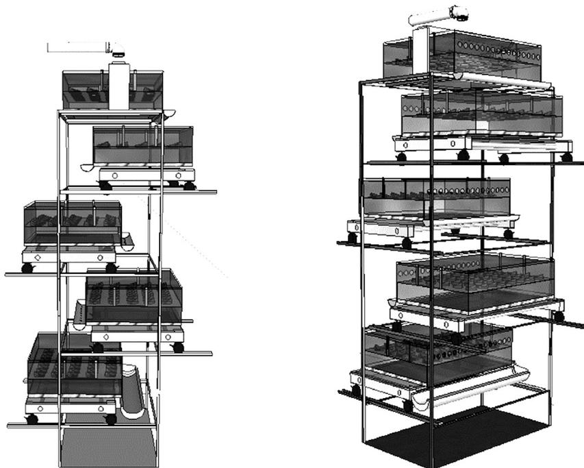
**Figure 7.** Conceptual design for the vertical flow treatment system, with the use of bivalves.
