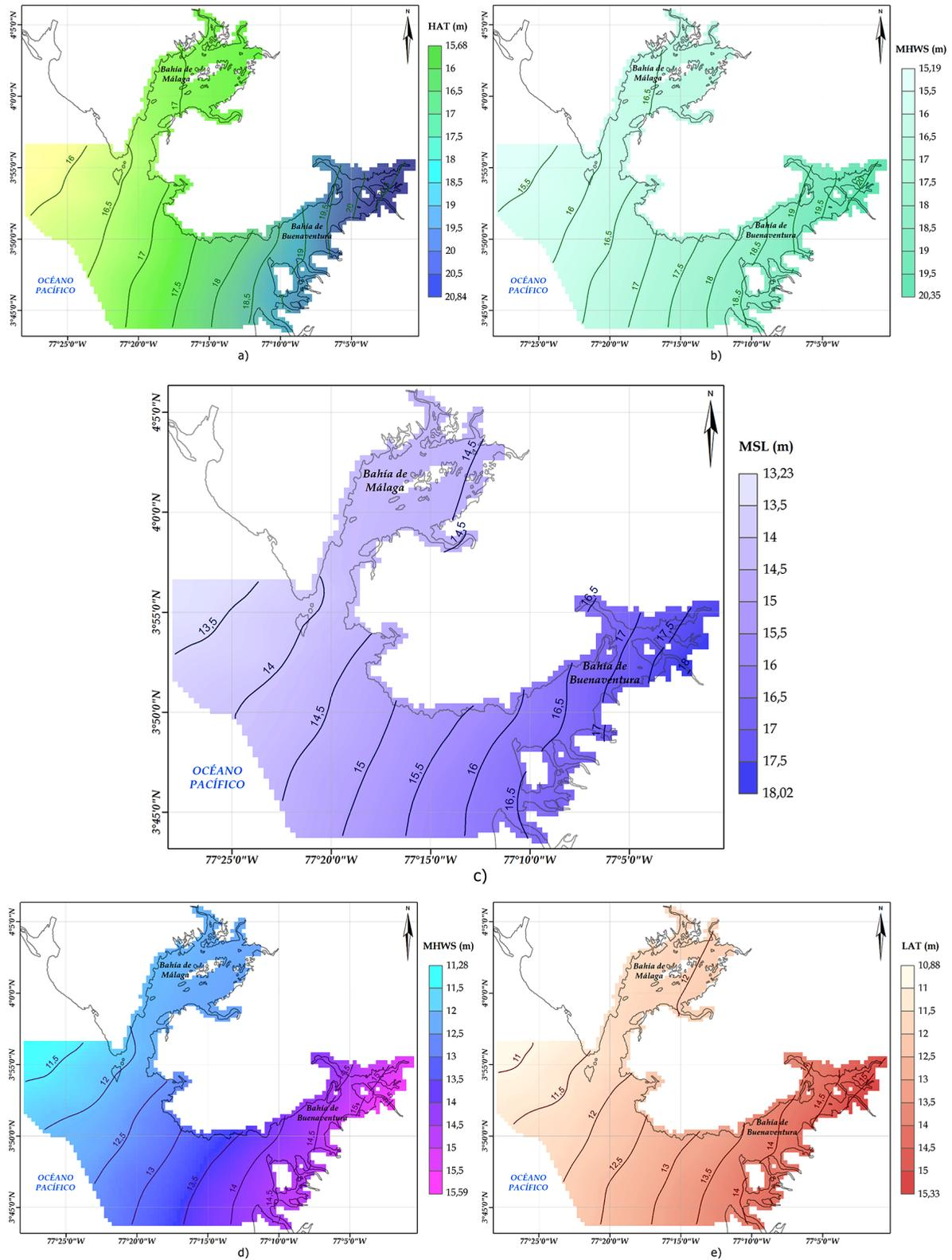
**Figure 4.** Surfaces of vertical datums referred to the WGS84 ellipsoid: a). Surface of the highest astronomic high tide. b). Surface of the average high syzygy tides. c). Surface of the average sea level. d). Surface of the average low syzygy tides. e). Surface of the lowest astronomic low tide.
