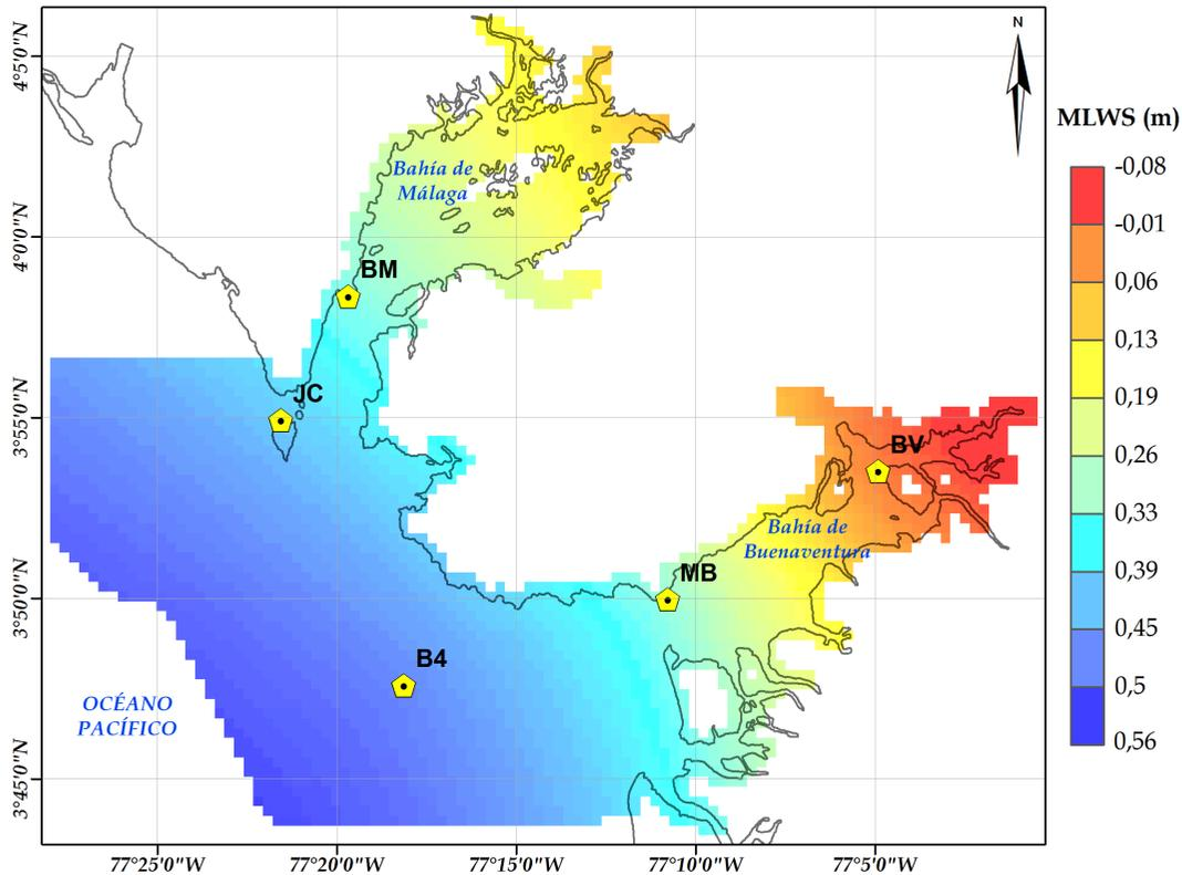
**Figure 3.** Tide gauge stations. Surface with relative heights referred to the MLWS=0 of the BV station in the Island of Cascajal in Buenaventura.
