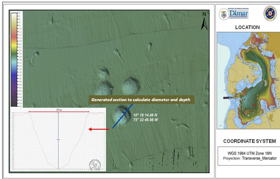
**Figure 3.** Details of the characteristics found in the muddy bottom of the southern area of the bay of Cartagena de Indias. Most of these pockmarks are around 20 m in diameter and are grouped or aligned to 3 meters deep as possible product of structural control in depth.
