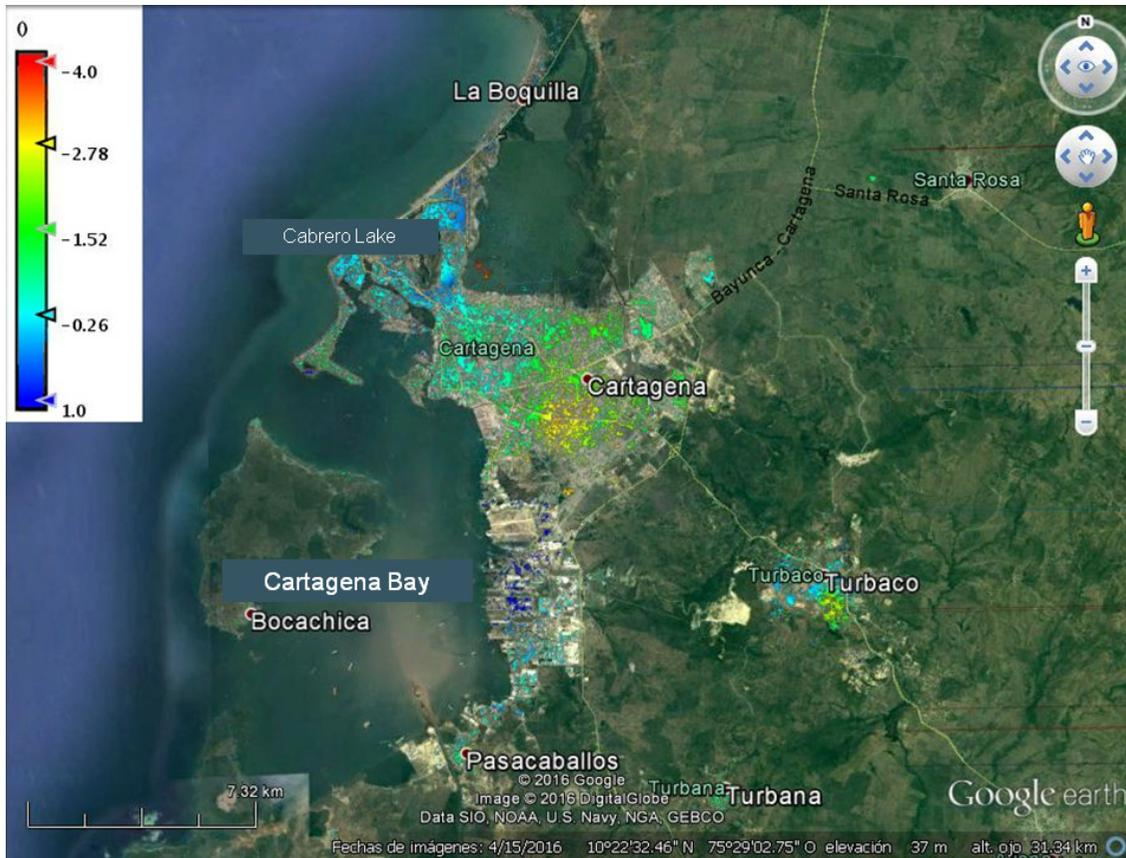
**Figure 8.** Interferogram for the period May 2015-March 2016 in the Cartagena area, the values (in millimeters) show the descend in the terrain in the year of observation.
