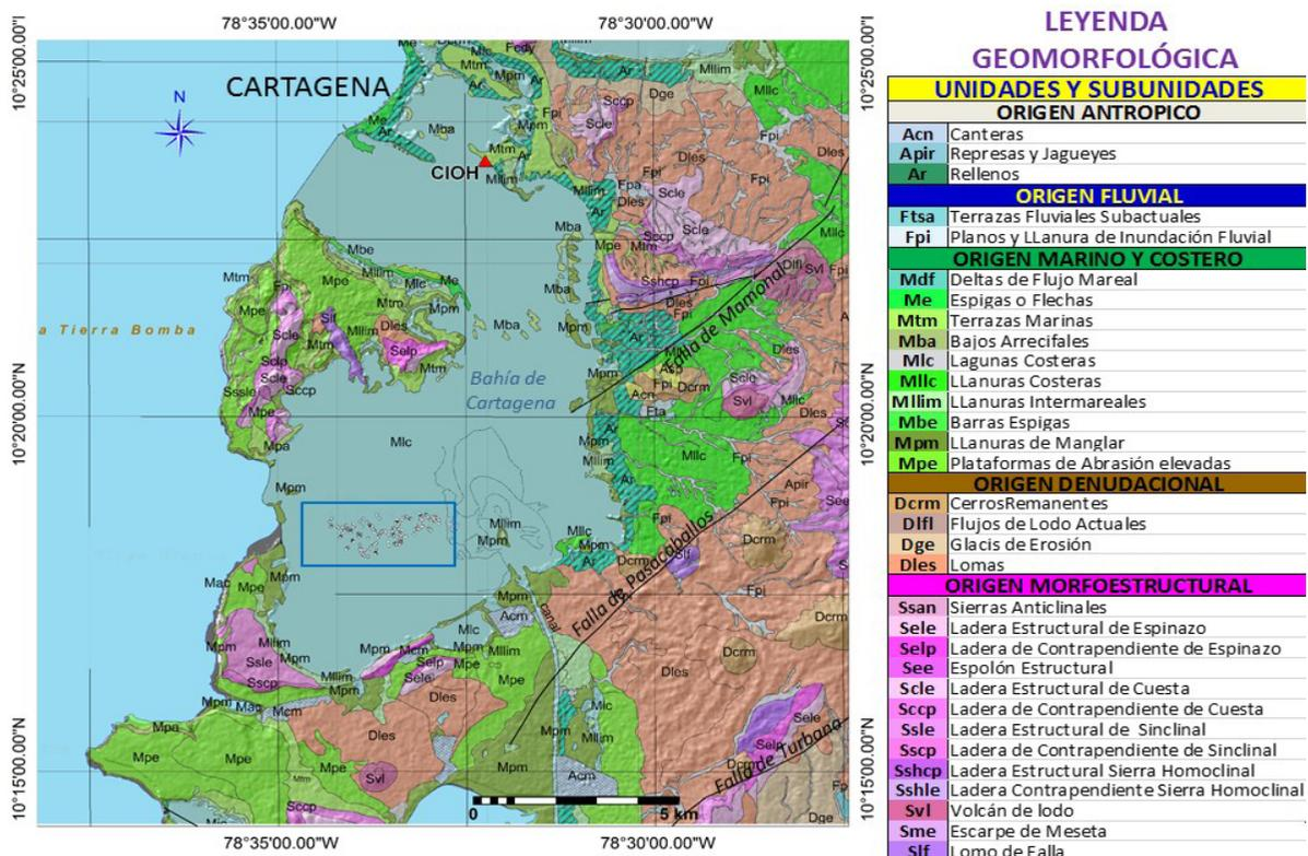
**Figura 12.** Geomorphological map of the bay of Cartagena surroundings. Note the blue box with the location of the submarine manifestations of mudholes and pockmarks and the plume of sediments brought to the bay through the Canal del Dique. Taken and modified by Carvajal (2017) & Andrade *et al.*, (2017).
