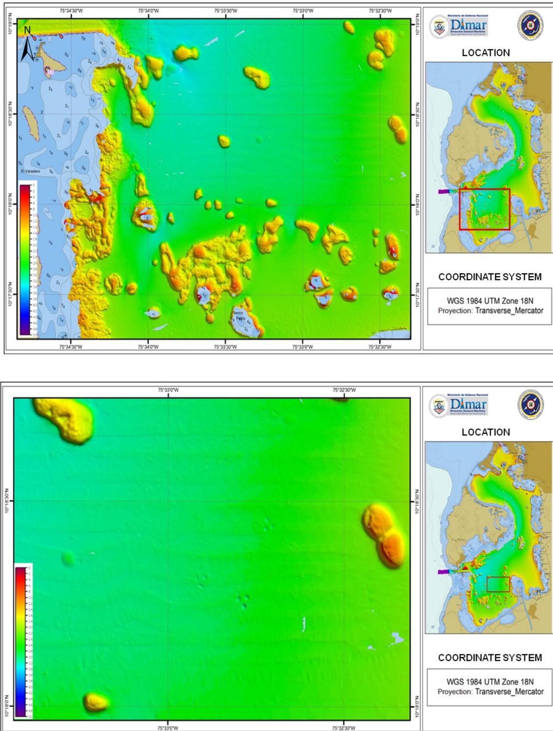
**Figure 2.** View of the multibeam survey in the southern area of the Bay of Cartagena. A relatively flat bottom (in green) is observed, dotted by elevations that rise abruptly almost to the surface, which is associated with old springs or mouths of mud volcanoes, several of which still conserve the upper crater.
