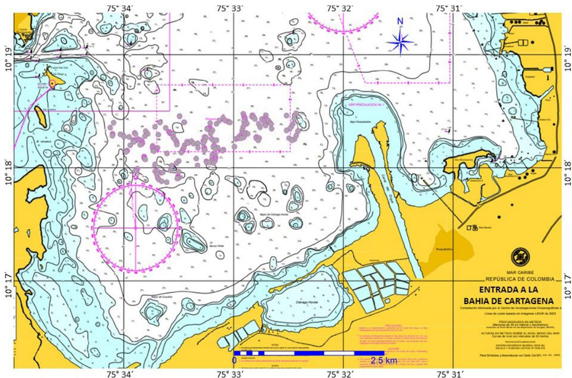
**Figure 10.** Bathymetry of the southern part of the Bay of Cartagena. Note both the distribution of the mud springs and "pockmarks" (grey circles) and the shallow reefs present in the sector, as well as the location of the mouth of canal del Dique by the SE sector (Taken and modified by CIOH 2011).
