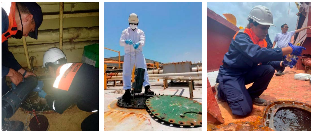
Figure 2. Microbiological sampling of ballast water on board ships
