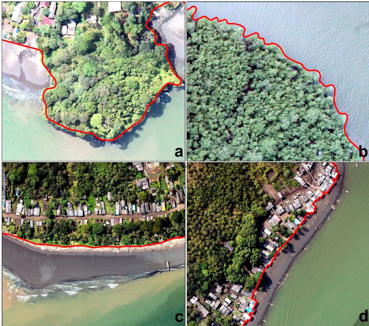
Figure 2. Criteria for digitizing the coast lines. a. Coastline defined by the cliff base; b. Coastline defined by the coastal edge of the mangrove in intertidal zones; c. Coastline defined by the landward boundary of a beach; d. Coastline defined by the edge of infrastructure.
