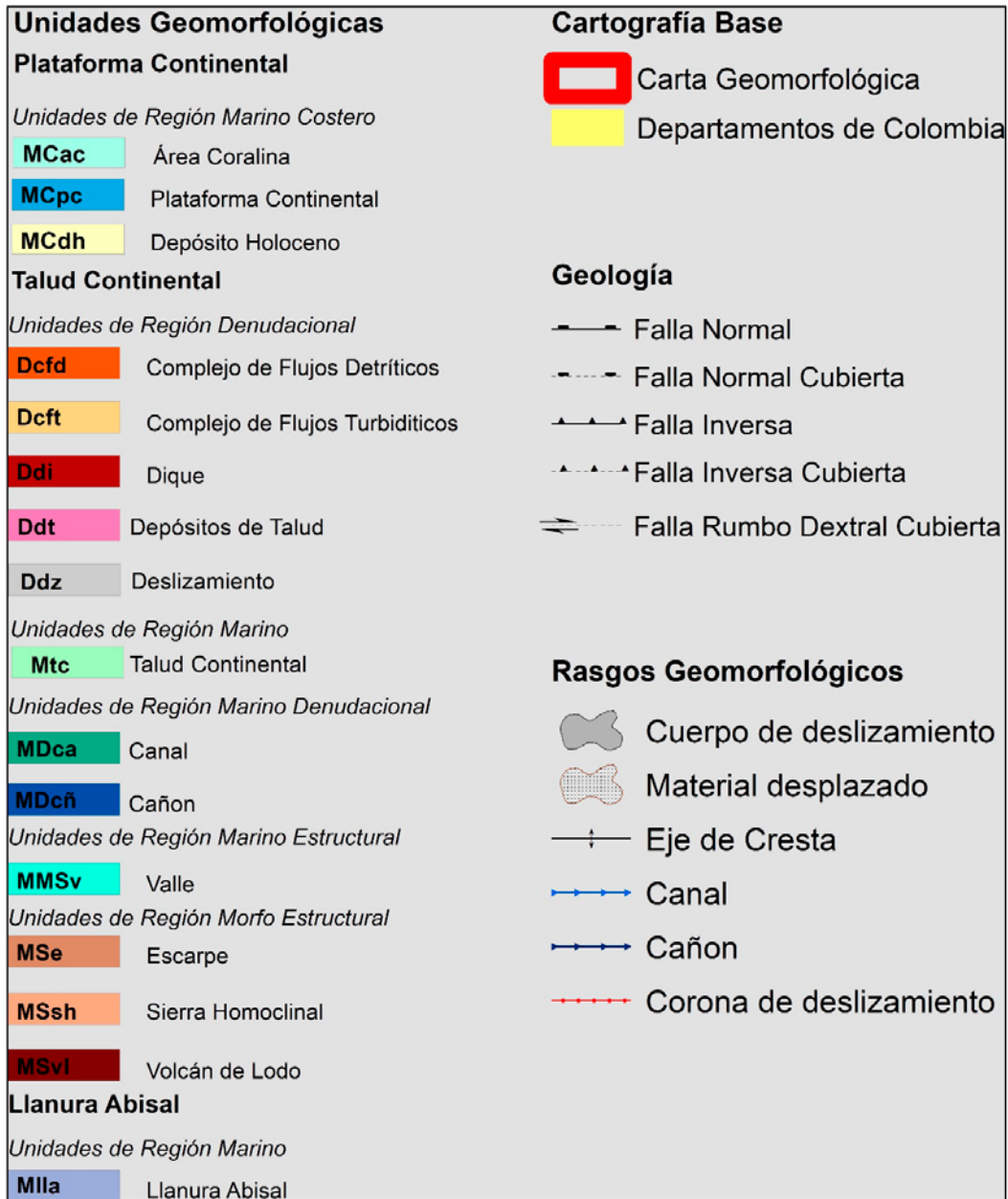
Annex 1 - Details of the geomorphological units and base cartography of Charts 1408 and 1409 showing the geomorphological units of the Colombian Caribbean Sea at a scale of 1:250 000.
